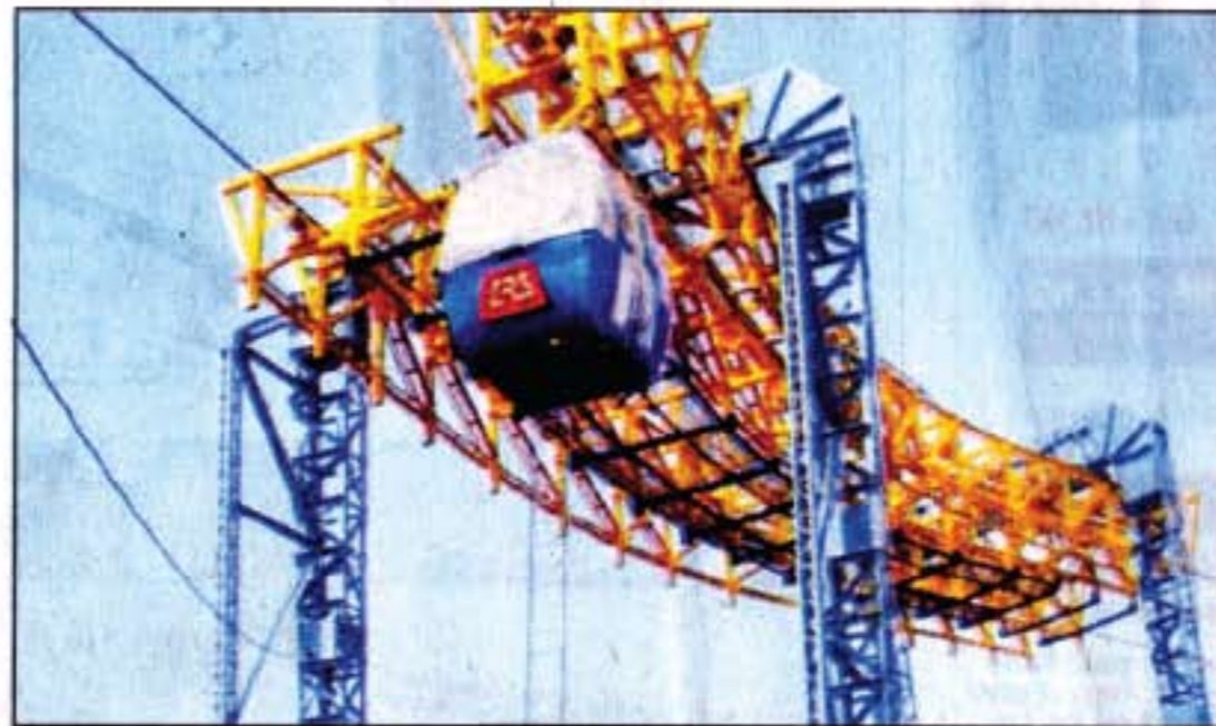
Curvo can travel at a speed of 12.6 km per hour by consuming 8-9 MW power
